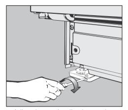
Adjust the rear leveling legs to the required height.
